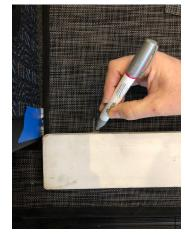
the board to the other side of the same L-track and repeat the marking procedure. You should now have a long skinny rectangular box drawn on the mat that will be used to indicate where to cut the mat.
