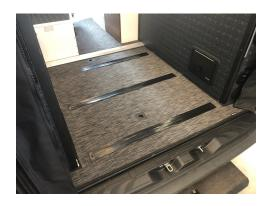
This tutorial explains how to <u>PERMANENTLY</u> modify your new cargo area mat in order to gain access to the existing L-tracks located in the cargo area of your Storyteller without requiring removal of the mat.
